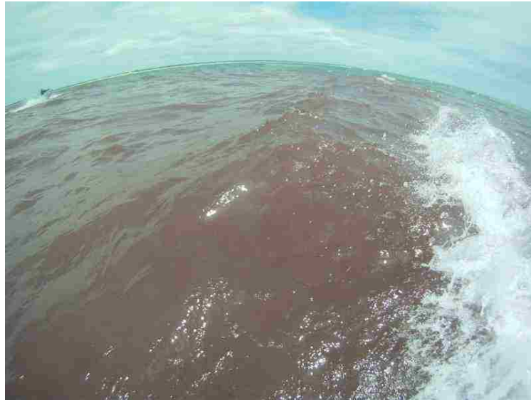
Figure 2.5: An example GoPro image with a breaking wave. The discoloration of the water surface was due to a rhodamine dye release earlier that day.
